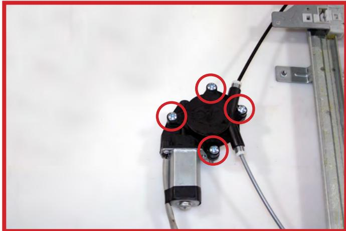
With the motor placed on the regulator install the new long bolts circled in red.
