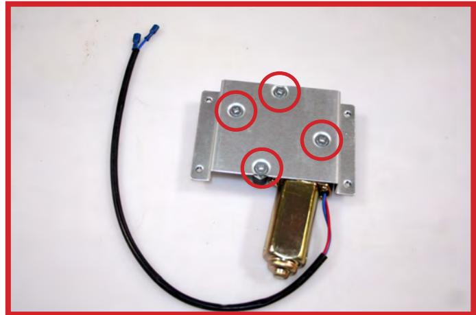
Remove the bolts circled in red to remove the motor from the mounting bracket.
