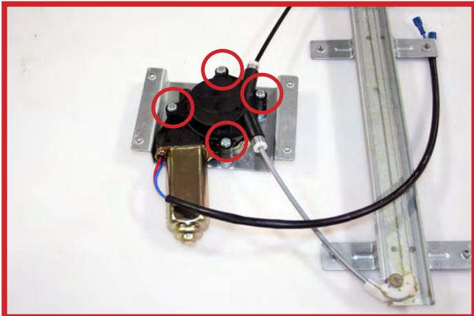
Remove the bolts circled in red. Separate the regulator from the motor using a flat blade screw driver.
