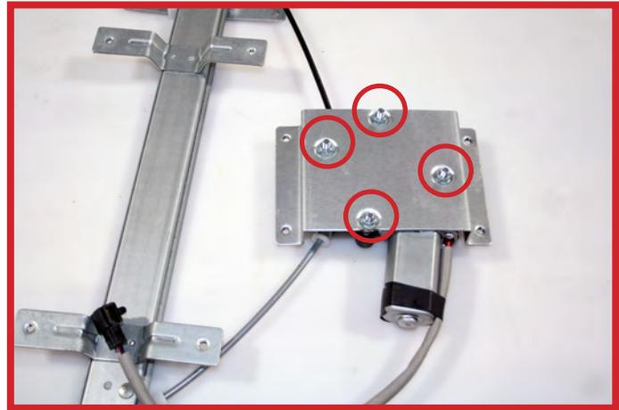
Turn the regulator over and place the motor mounting bracket onto the long bolts. Install the nylock nuts evenly circled in red.
