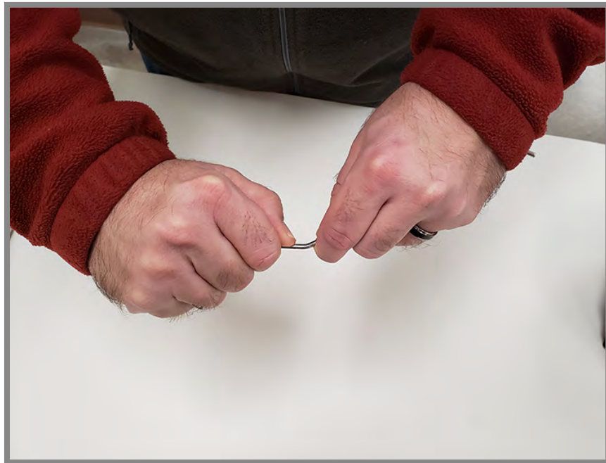
Using two hands, bend the clip inward. Repeat before each use to avoid clip loss.
