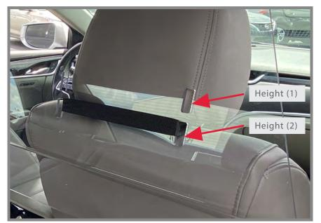
There are two installation holes for optional drivers height adjustment:
