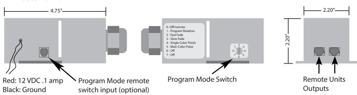
Install the Master Unit in any location with a simple two wire hookup. The Master Unit can be used alone or with additional Remote Units. To add Remote Units simply plug a cable and Remote Unit into either or both outputs of the Master. This output will power the Remote Unit and the selected program mode of the Master Unit will determine the program mode of the Remote Units.
