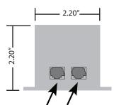
Either port can be used for: Input from Master Input from Remote Unit Output for additional Remote Unit
